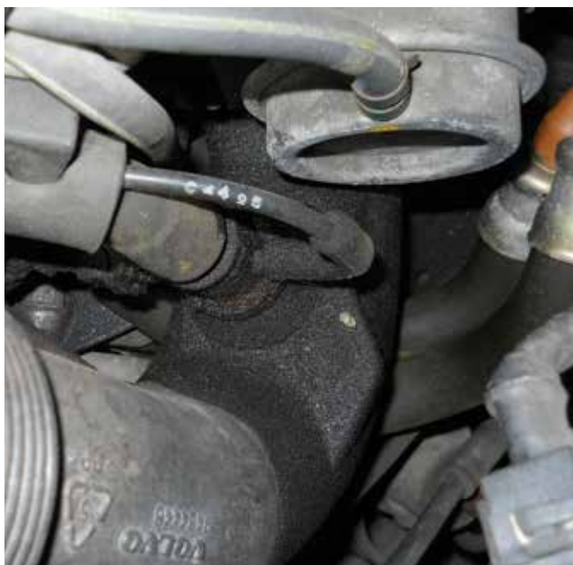
Here's the heater element for the PCV system on a 1997 850 Turbo. The electrical connector can fill with oil and cause a short.
