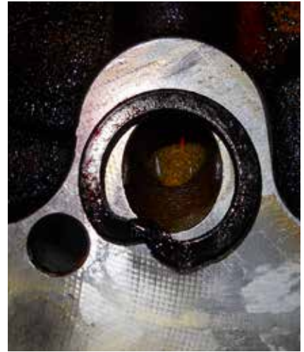
Always change all of the oil seals when you remove the pan.
