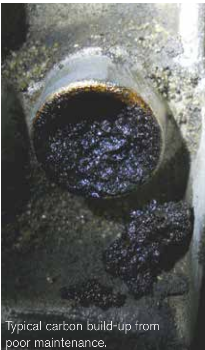
This is where the PCV gets its vacuum, and it's where the trouble starts. If caught early enough, you can get away with just cleaning out the hole.
