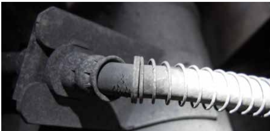
As Volvos and all other makes age, the brake hydraulic hoses will start to develop cracks. If left to continue to deteriorate they can become a serious safety hazard. The hoses for front calipers wear faster than those for the rear because of the constant flexing when the wheels turn.
