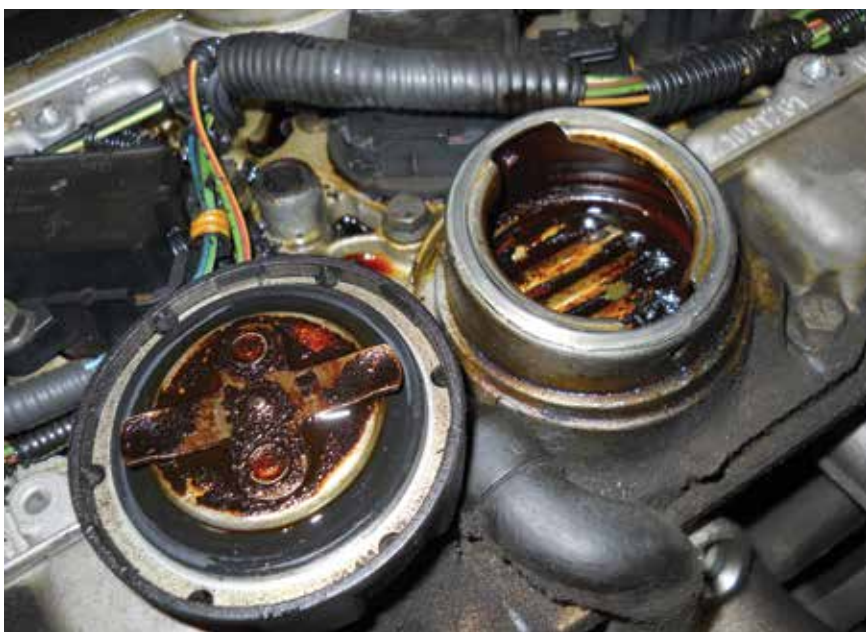
The carbon and oil sludge buildup on this Volvo's oil filler cap is a sure sign that this car has not seen regular service.
