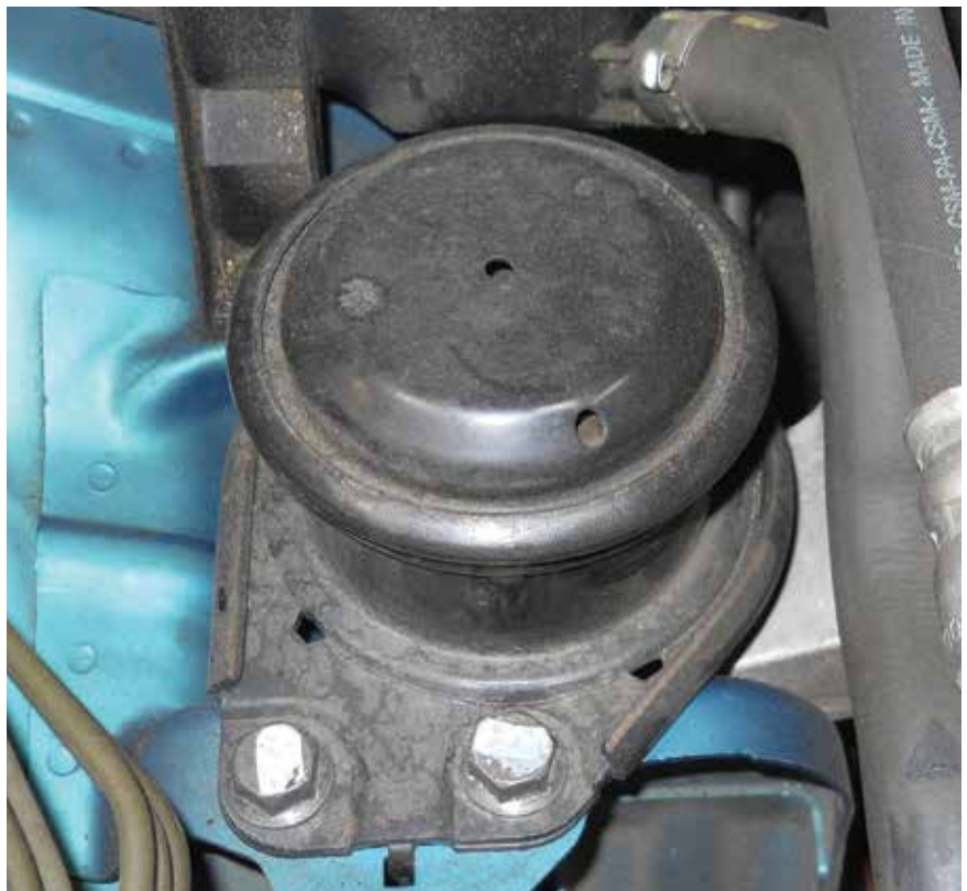
Hydraulic motor mounts make for smoothness — until they lose their fluid.
