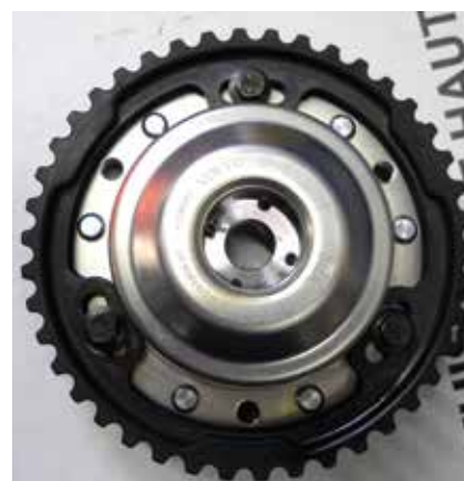
The new CVVT hub has no timing marks, but with the cam lock installed you don't have to worry about that.
