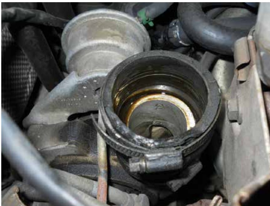
This short intercooler hose on top of the turbo will crack if the hard plastic pipe that connects to it is moved too far without loosening the clamps.
