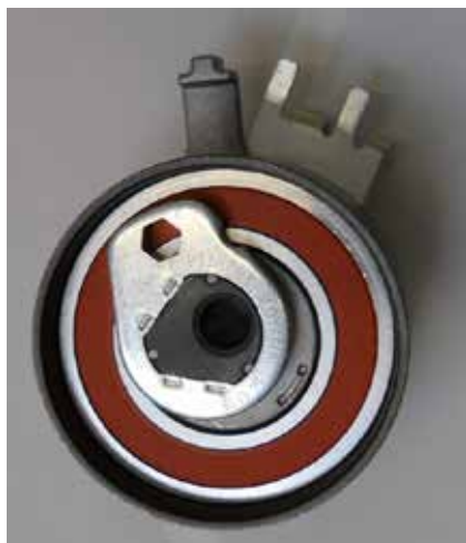
Here's the mechanical tensioner from a Volvo B5254T engine.
