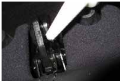
Move the lever several times in the lock or unlock direction and apply lubricant to the latch/operating lever.
