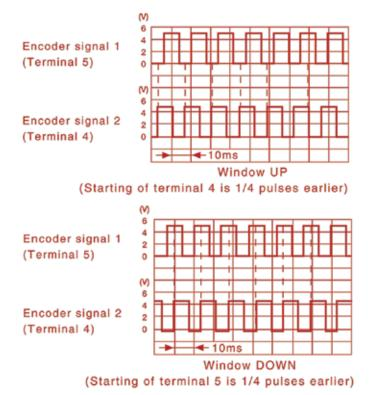
The encoder signal from the main power window switch should show an on-off square wave pattern that alternates between zero and five volts. Differences between the patterns relate to whether the window is going up or down, and which pin (signal) is being monitored
