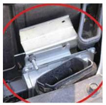
Pre-scanning for trouble codes may show that the ECM mounted in front of the battery on this 2015 Rogue® has suffered internal damage and must be replaced. Even if the ECM suffered no collision-related damage, post-repair scanning will detect if disconnecting and reconnecting any devices during the repair process has led to an inability to communicate properly with the ECM.
