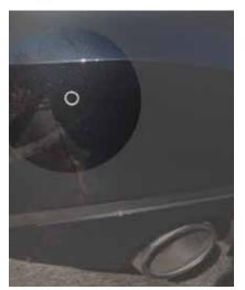
Electronic sonar sensors in Nissan front and rear bumpers are engineered to exact positions within the fascia. Aftermarket and recycled fascia may not meet the same specifications, and if the imaging technology cannot be properly located, may not function as intended.
