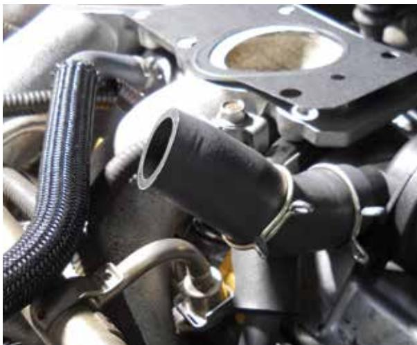
Make sure you order the PCV valve and hoses when you perform the valve cover job. The hoses always crack, and replacing the valve is always a good idea when repairing oil leaks.
