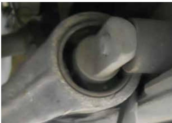
This is the standard test procedure for checking the control arm bushings on a Volvo. When they are really bad you can feel the wheels jerking back when stabbing the brake pedal at low speeds.
