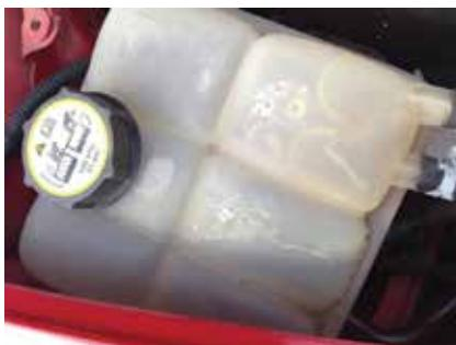
The coolant tanks on the P1 cars tend to crack along the gap in hood where sunlight can expose it to UV rays.
