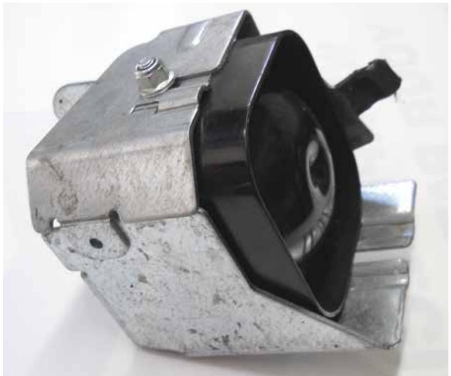
In the image you can see the alarm module removed from a 2001 Volvo V70XC. The internal rechargeable battery has failed causing intermittent alarm malfunctions.
