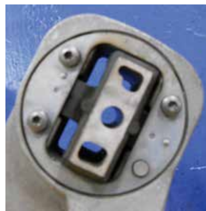
Worn or broken engine torque mounts can make shifting feel unduly harsh.
