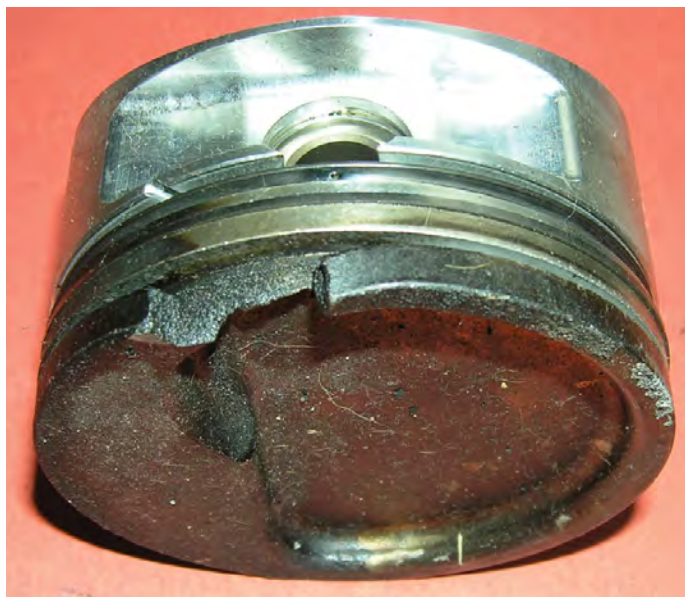
Low octane fuel combined with too much compression or spark advance can lead to serious engine damage.
