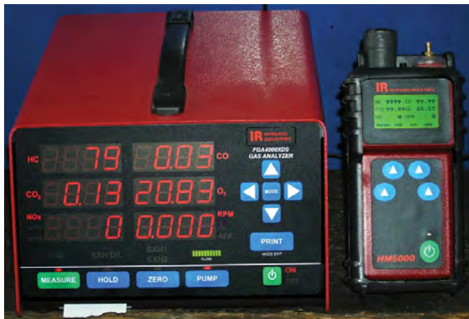
The NOx reading on this portable 5-gas exhaust analyzer is an indicator of detonation.
