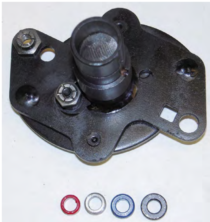
An MSD distributor includes an assortment of bushings and springs that can be used to change the rate and limits of spark advance.
