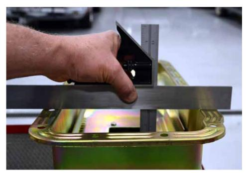
One measurement that should always be performed is the pan floor-to-oil pump suction distance. There are a couple of ways of doing this, and I generally do both: a physical measurement with a square and straight edge, and a double check with clay.
