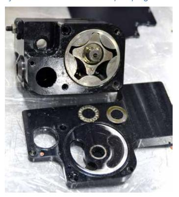
elements are located off center and they generate uneven pressure loads that can make them vibrate and shake the drive system. Increasing volume is as simple as increasing the drive and driven element length, but they don't like to digest things that aren't oil.
