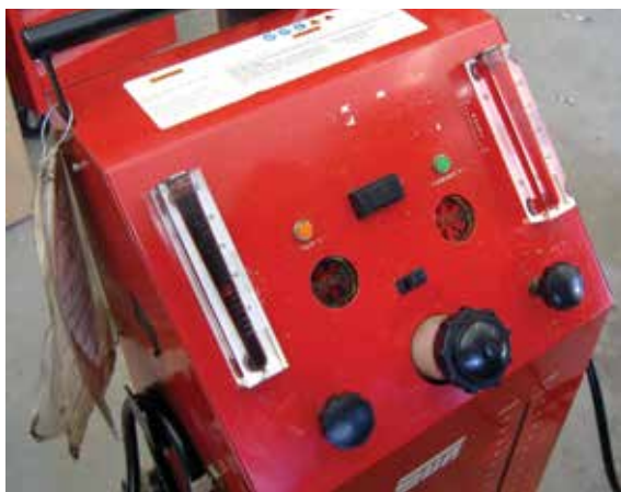
Regular transmission fluid maintenance is much more expensive with synthetic ATF than it was with conventional Dexron, but transmission work is much more expensive, too. The visual comparison of clean to dirty ATF as seen on this flush machine is a powerful customer pleaser.
