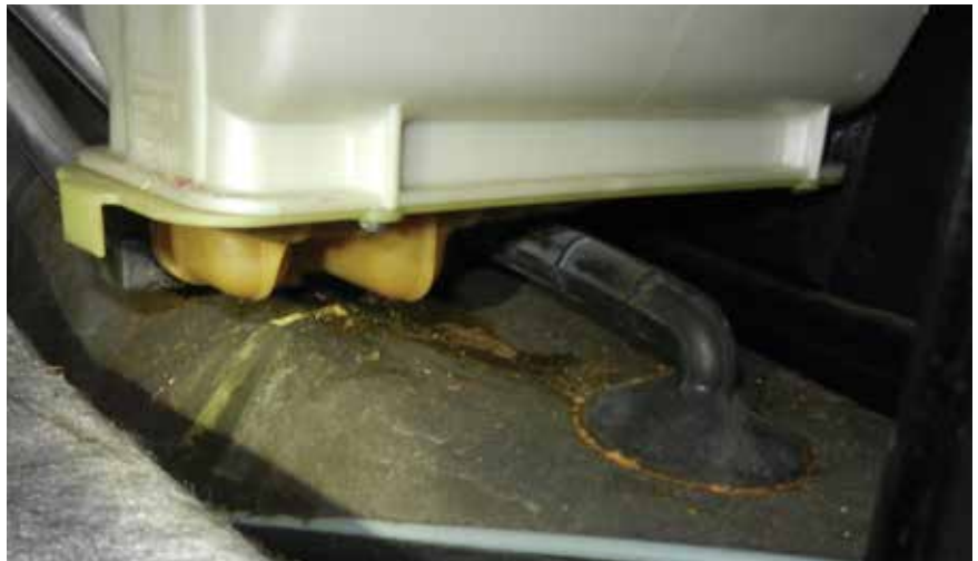
The most common heater core leaks seen at independent shops are those from the 1993-2000 Volvo 850/70 series cars.
