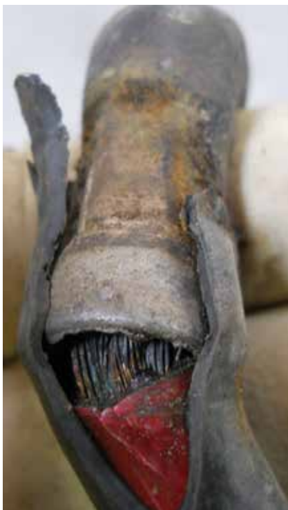
The positive battery cable can corrode inside the clamp's crimp, causing intermittent high resistance.
