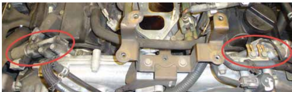
The intake valve timing (IVT) control solenoid valves are located on either side of the front of the engine block. The bank 1 IVT control solenoid valve is on the passenger side.
