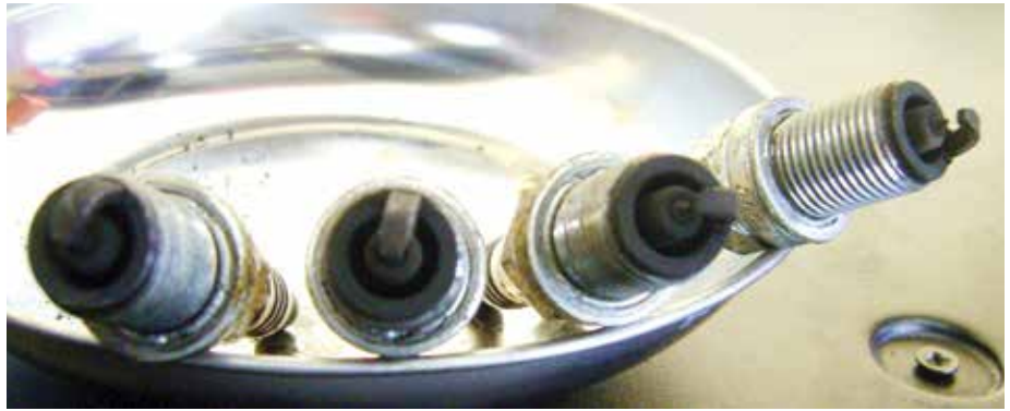
These plugs are clearly getting too much fuel, yet the fuel trims on this 1997 Maxima still showed a lean condition.
