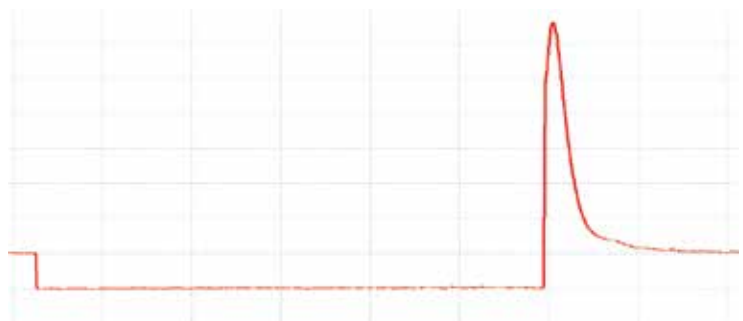
In some instances, there won't be a pintle hump reflected in Nissan injector control waveforms.
