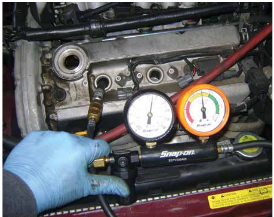
At 300K miles this engine isn't going to get the mileage it once did. With air hissing in the crankcase it's going to need a rebuild to get its former glory back.
