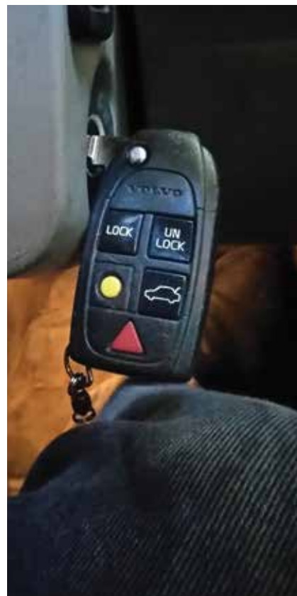
A floppy key can be a safety issue, because it can hang down, close to the driver's knee, which could cause them to inadvertently switch off the engine while driving.
