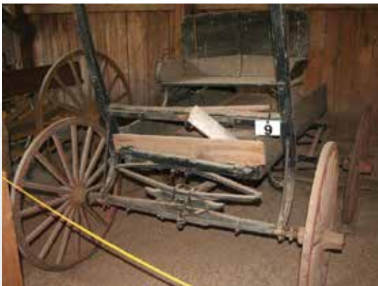
Note the springs isolating the carriage from the axle and wheels.
