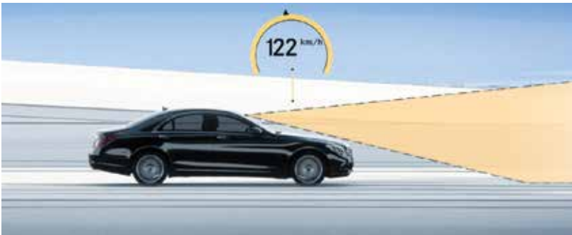
Stereo cameras “see” the road allowing the suspension to adapt ahead of time.
