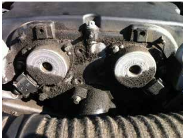
These solenoids have been leaking for too long. They will have to be cleaned and evaluated for the leak source.
