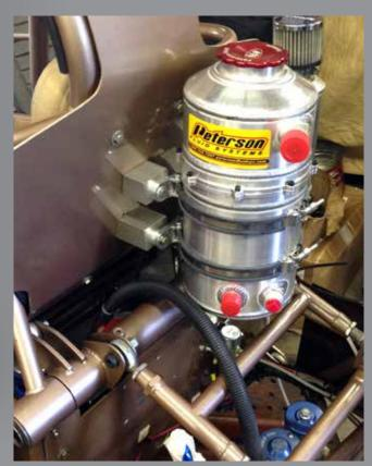
quantity of oil, but bigger is better, within reason. Oil tanks should be filled to about 2/3 full and checked with the engine running to allow sufficient head space for de-aeration. If you're using a remote breather, make sure to mount one large enough so it is at least as high as the oil tank breather fitting and check it between runs for oil carryout. Tanks may or may not have an integral breather welded
