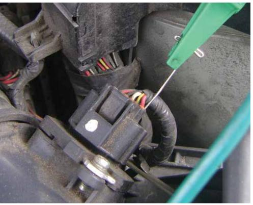
Back probing the MAF signal gives us info directly from the sensor. If the voltage differs from the data stream on the scanner, we know we have a resistance problem in the wire harness or ECM connection. If we can change the data by moving the harness we know where the problem is.
