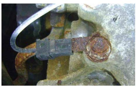
This Quest has been crippled by rust. After cleaning the mounting and replacing the terminal on the wire, it's time to check the rest of the grounds on the van for the same problem.
