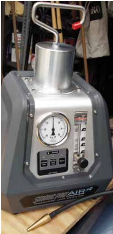
A smoke machine is great for finding intake leaks, and we've even identified a burned-through piston with one.
