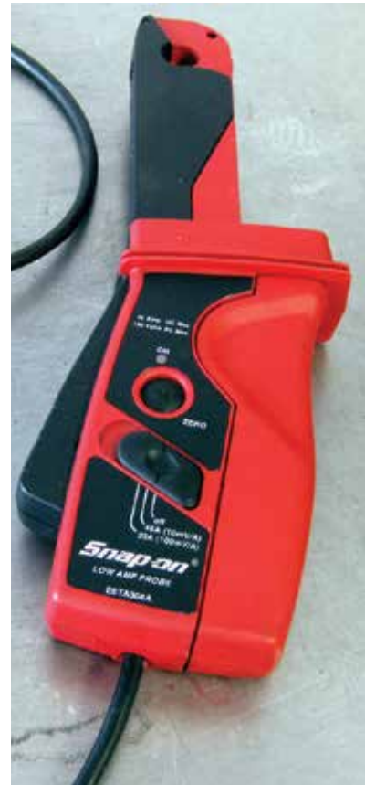
A low-amp inductive probe that works with your DMM or lab scope allows you to read small currents without breaking connections.
