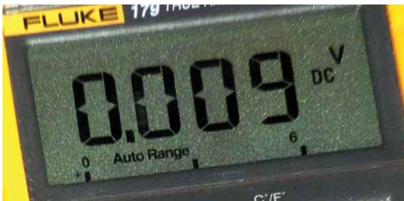
This is the kind of reading you should like to see when checking voltage drop in the pump’s ground.
