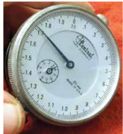
A worn-down cam lobe can prevent sufficient filling or exhausting of a cylinder. You can check for proper lift with a dial indicator on a suitable fixture if you suspect such a condition. Also, look for a collapsed lifter.
