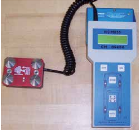
Measuring ride height is critically important since ride height determines the specific alignment settings. Mercedes-Benz dealers use this ROMESS gauge along with their precision MKS alignment rack to ensure the highest levels of accuracy.
