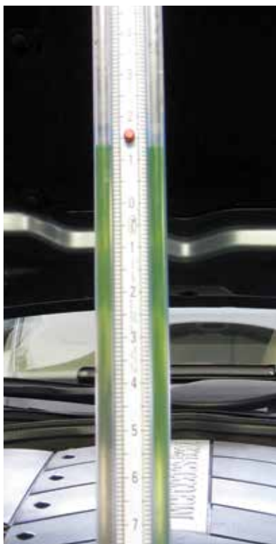
You can check crankcase ventilation pressure with a manometer.
