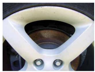
Rust on the rotors means this car hasn't been driven in a long while. If nothing is obviously broken you may want to put some miles on it before you try to diagnose suspension noises.
