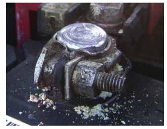
Customers may not be concerned about the things they should be concerned about. Having to frequently jump start their car because of a loose and corroded battery terminal wasn't important until it caused them to fail their emissions inspection.
