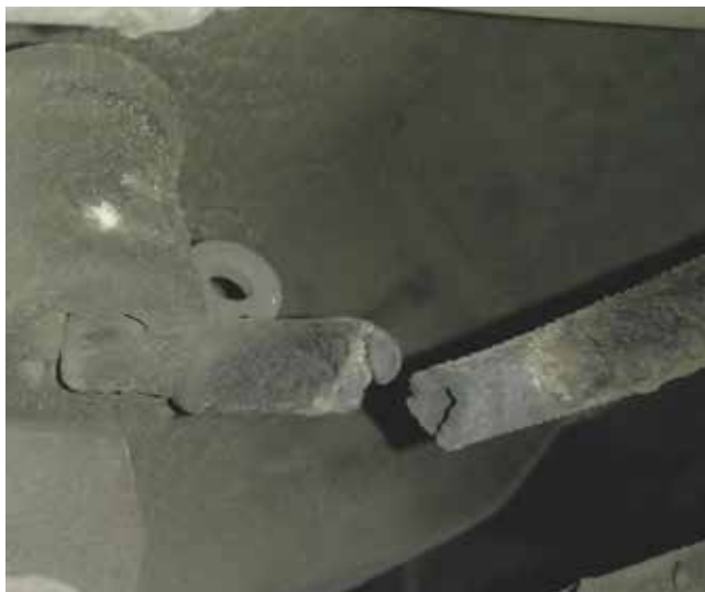
Cracked hose at roll over valve.
