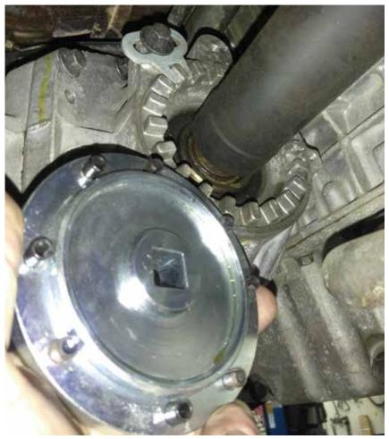
The one tool you should have in the shop when working on the Volvo angle gear is Volvo special service tool 9995371. This tool is the only way to get the pre-load adjustment nut off without damage.
