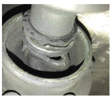
During your regular inspections, check the slip yoke boots for damage. If a boot is torn or damaged, the slip yoke or yokes will probably need to be replaced soon.
