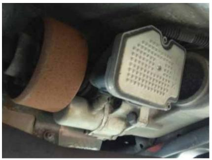
Volvo started using various versions of the Haldex electronically controlled rear differential starting in 2001 instead of the viscous coupler type.
