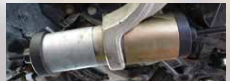
Replacing bushings can be quickly done on the car with the proper tools.
