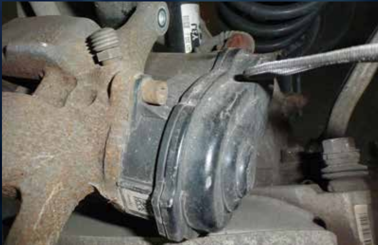
The actuator is a simple bolt on design attached to a modified brake caliper.
