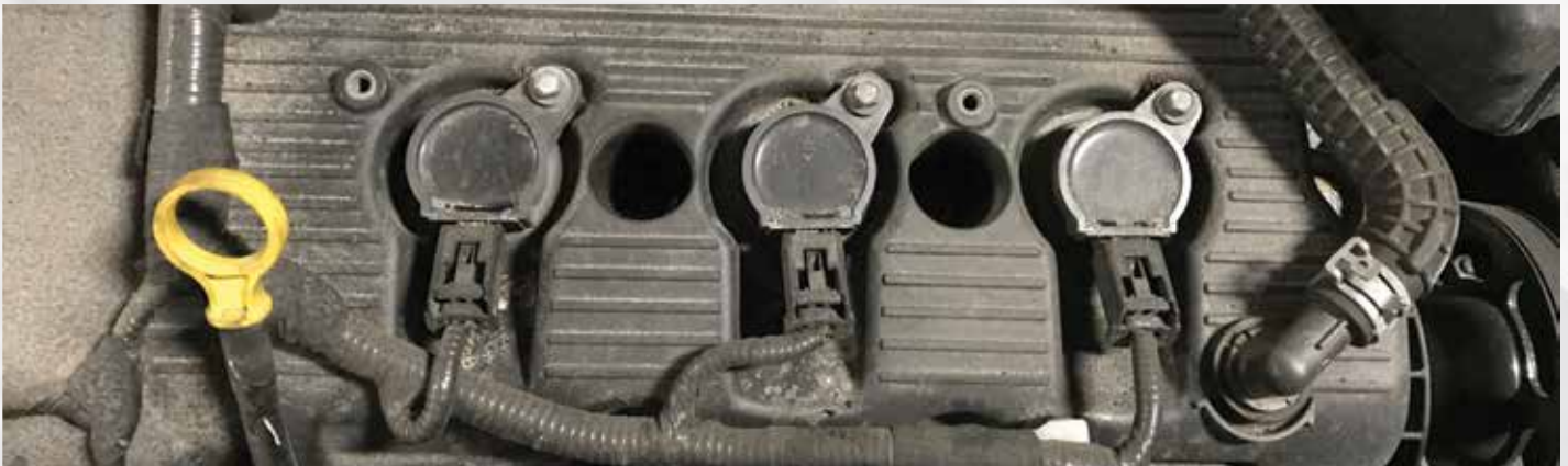
Half of a V-6 engine shows one coil for each of the three cylinders. This allows enough time for thorough coil saturation.
