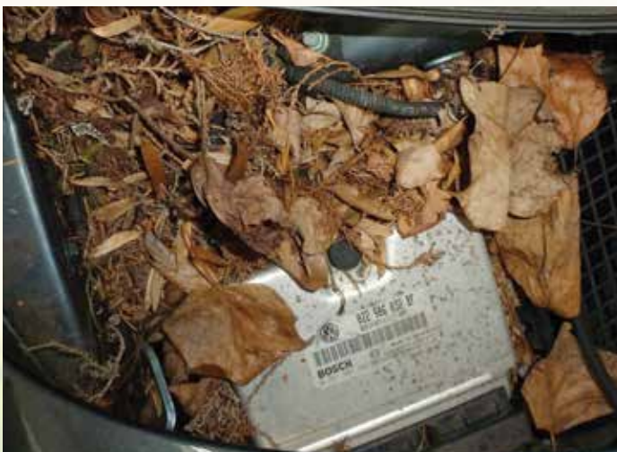
If not periodically cleaned, the cowl area will eventually clog, leading to water ingress.
