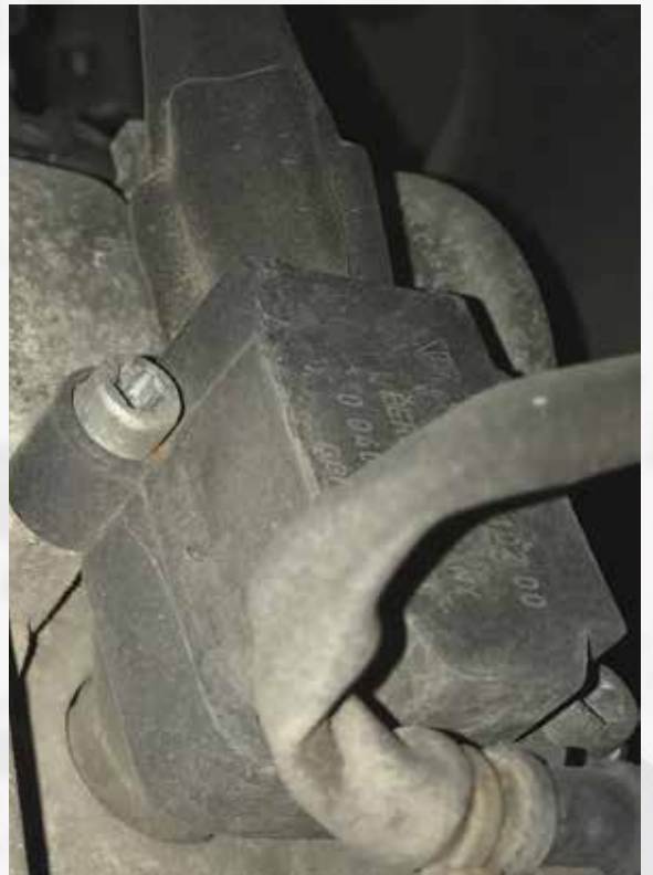
How's this for a bad environment? This coil has to live under the engine where all the water, ice and road salt can attack.
