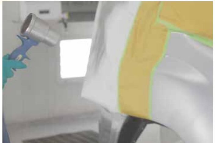
Portable air blowers are significantly less costly to operate than increasing the heat in your booth bake cycle.
