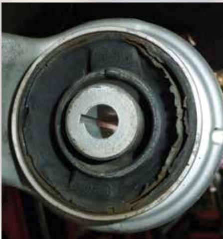
This lower control arm bushing has failed, allowing excessive wheel movement and noise.
