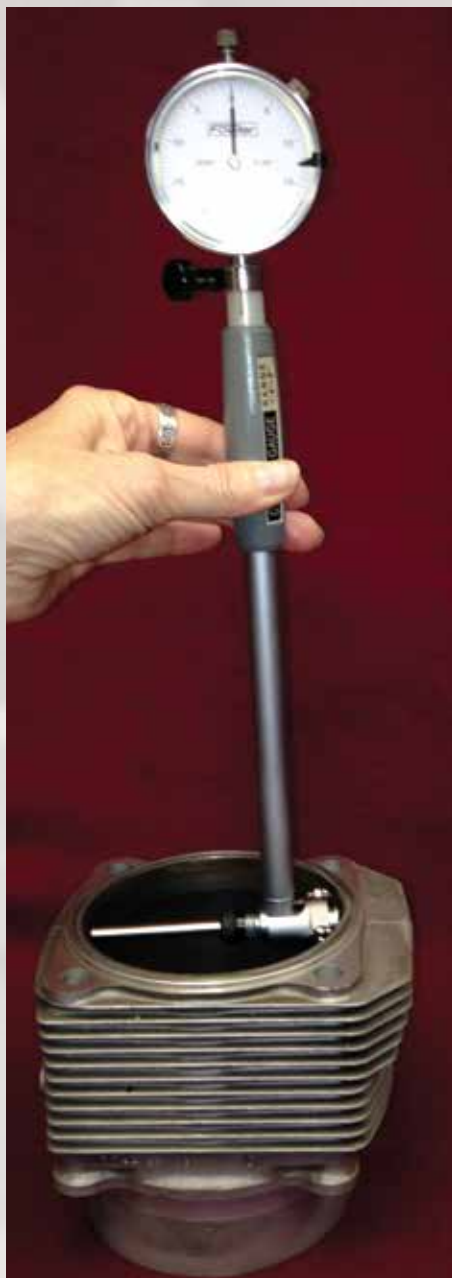
Always follow the manufacturer's procedures for measuring any engine component. This cylinder is being assessed for reuse, and should be measured at several different points for roundness and taper.
