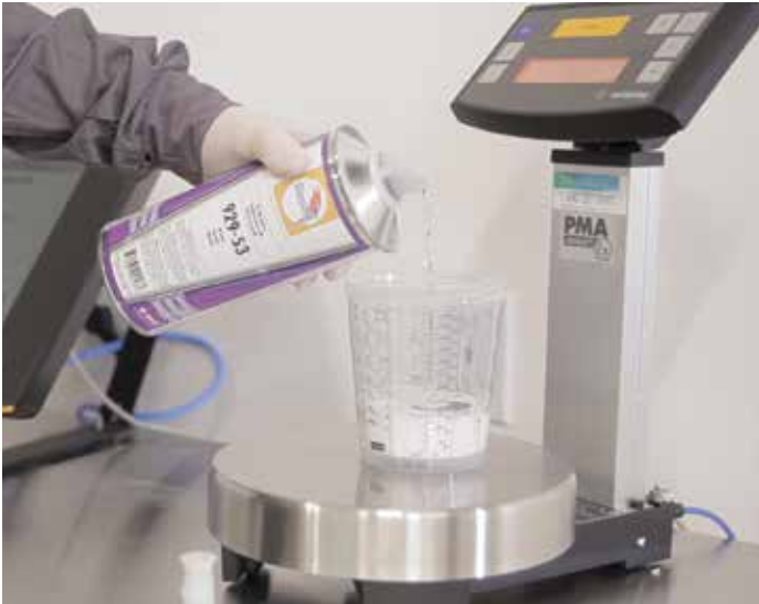
This painter is adding Glasurit 929-53 hardener to a mix of a 2 component Glasurit Urethane Sealer to create a ground coat color formula. The resulting gray ground coat enables poor hiding colors such as reds and yellows to achieve coverage and excellent color match with fewer coats.
