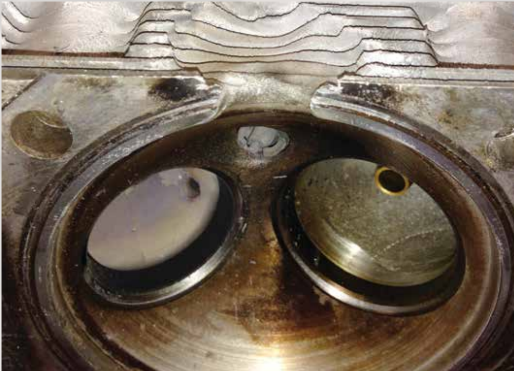
This turbocharged engine got too hot! Lean fuel to air ratios can turn an engine into a very expensive plasma cutter! Note the melted cooling fins on the side of the cylinder.
