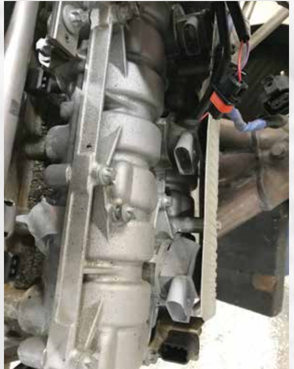
Were it not for the fact that this engine is out of the car, one would not be able to even see these coils. Servicing coils and plugs on this engine requires removal of exhaust components, heat shields and whatever else happens to be in the way.
