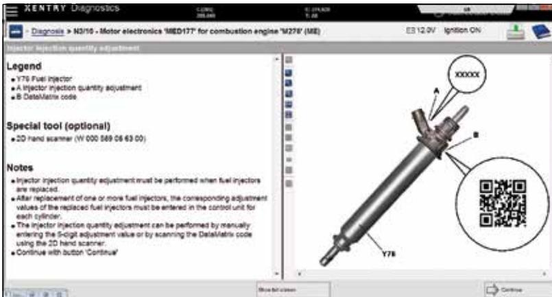
Programming isn't just limited to software updates: Modern fuel injectors need to be married to the engine control unit in order to work right. For this you need the special 2D code scanner as well as XENTRY.
