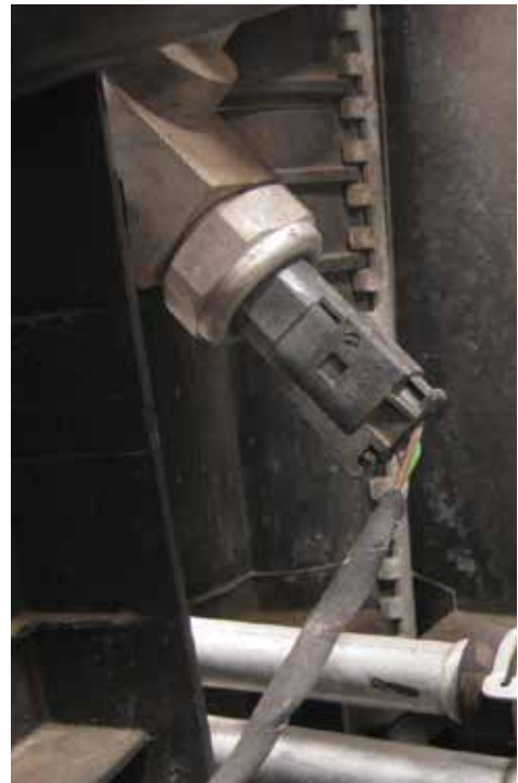
The refrigerant pressure sensor is usually located between the compressor and the condenser.
