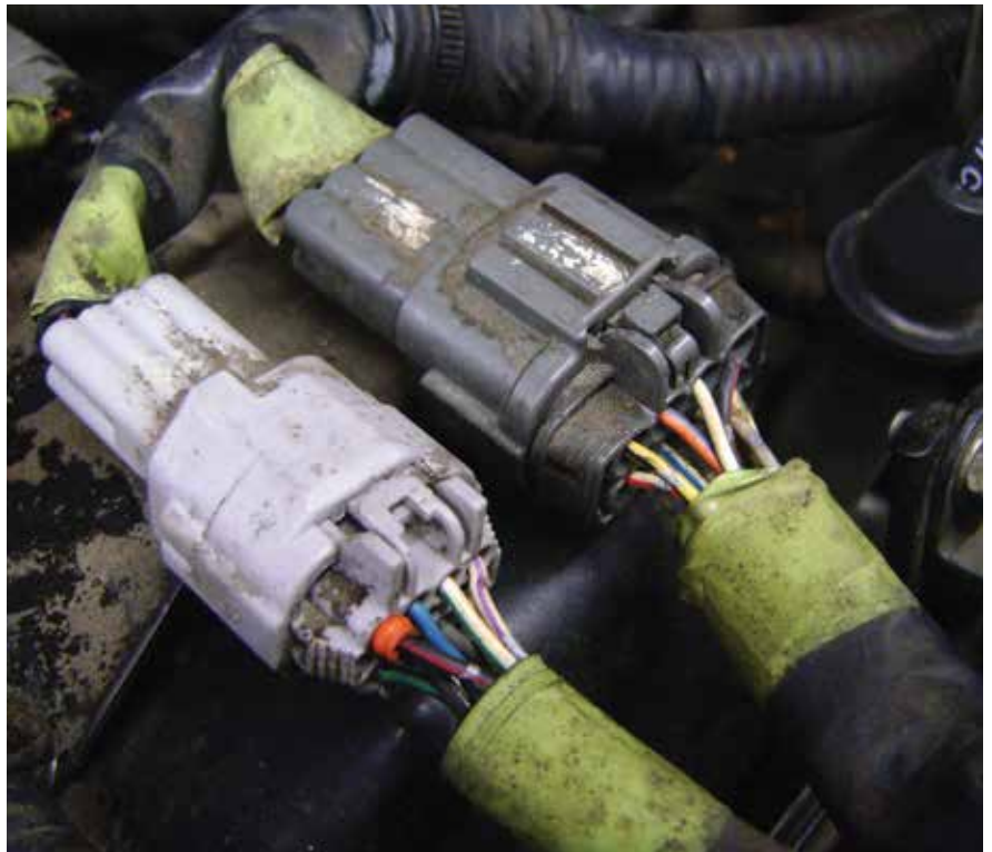
On the front of the right valve cover this fuel injector harness connector is the perfect place to test the electrical integrity of all the injectors quickly and easily.
