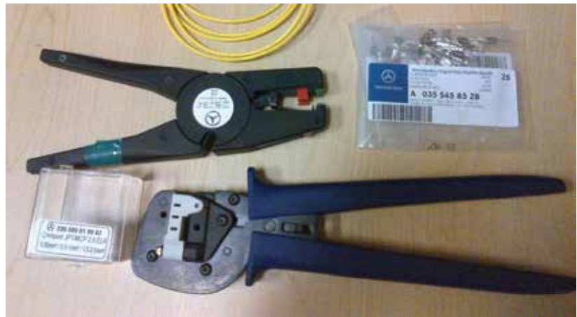
The Mercedes-Benz crimping tool (bottom) with the crimping die set for the JPT/MCP family of contacts installed. You can also see the automatic stripping tool, a bag of electrical contacts, and some repair wire.
