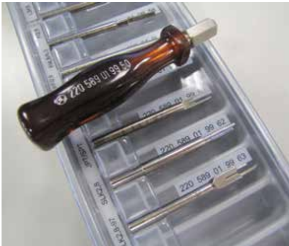
A few of the unpinning tools. The handle is universal; the tools themselves fit into the handle. Look closely and you can see that the 220 589 01 99 62 tool is for unpinning the SLK 2.8 family of connectors. Individually, the tools are relatively inexpensive. We have some of the common ones here in the shop, the rest we can borrow from our dealer.
