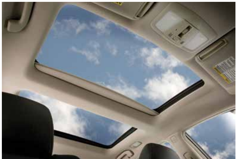
The 2011 Maxima was introduced in the US market with both a single and a dual panel sunroof option.
