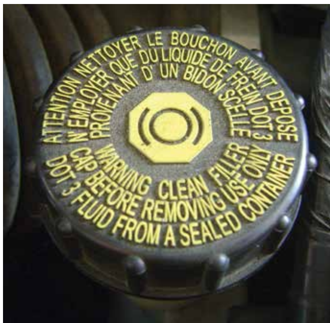
There is little variation in what fluid goes in the master cylinder of any street car and yet it's still labeled clearly "DOT 3."
