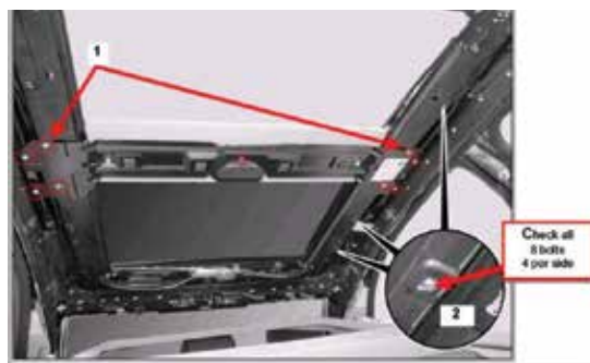
Replace any missing bolts, tightening all nine bolts to 5 Nm \pm 1 N.
