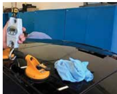
Hook a force gauge onto the cable tie and pull upwards with 25 kg or 50 lbs. of tractive force.
