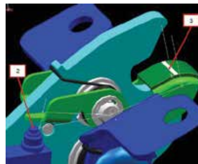
Apply lubricant (A000 989 36 60) to the lever.
