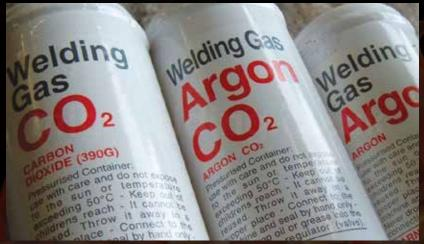
Different shielding gas types are required depending on whether you are welding steel or aluminum, the plate thickness, the type of wire electrode you are using, and other variables.
