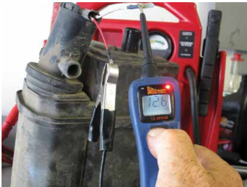
A good way to check an evap solenoid valve is by injecting 12V to see if it works.
