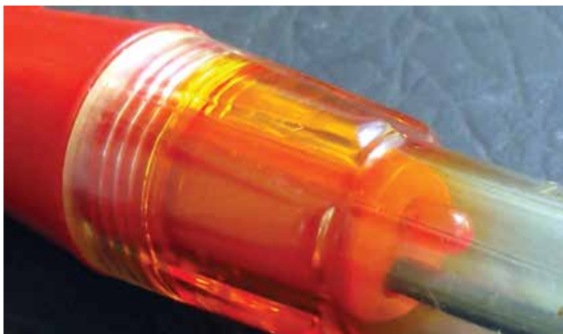
...always use the LED type as the old-fashioned incandescent-bulb variety can draw enough current to damage electronics.
