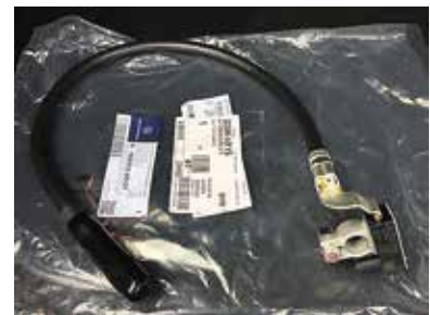
Here's what the Intelligent Battery Sensor looks like...
