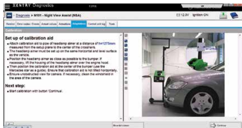
To calibrate a Night View Assist camera, which uses infrared light to display an image on the instrument cluster display, you need both a headlight aimer and the special calibration target. The XENTRY software walks you through every step of the procedure.
