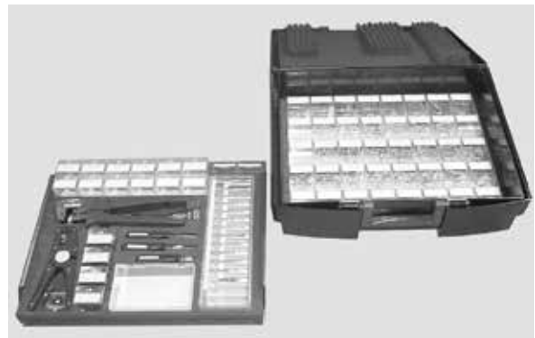
This is the basic harness repair kit. It comes with the crimp pliers and several die sets, wire strippers, and several unpinning tools. Also included is a carrying case and about 40 empty boxes to store connector pins. The supplementary car kit includes crimp sets and unpinning tools used in cars.
