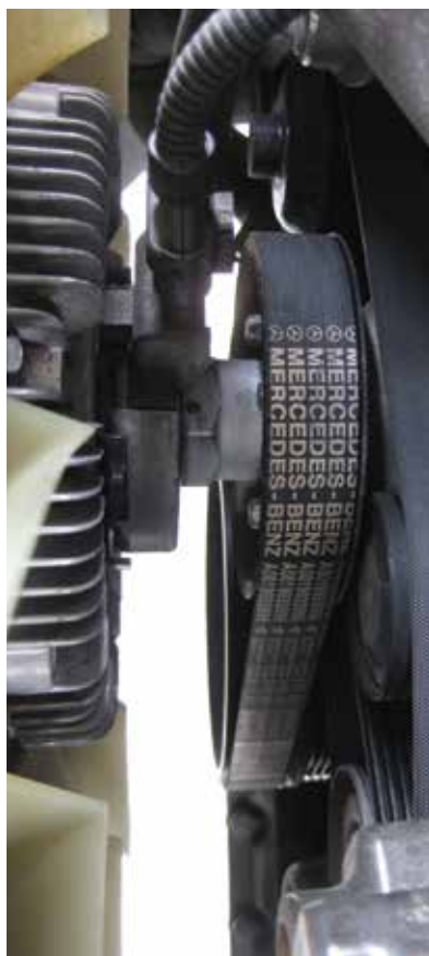
The electronically-controlled fan clutch went a long way in increasing efficiency and keeping the fan from spinning when it's not needed.
