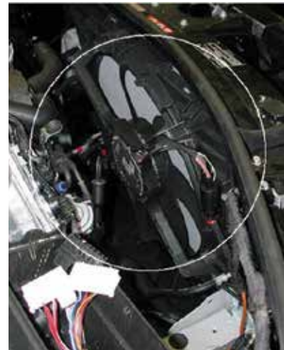
A typical later-model cooling fan and integrated suction fan control module.
