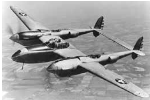
In WWII, turbocharging gave many of our warplanes, such as this Lockheed P-38 Lightning, superior performance at high altitudes where the air is thin. (Courtesy Airforce Image Gallery.)
