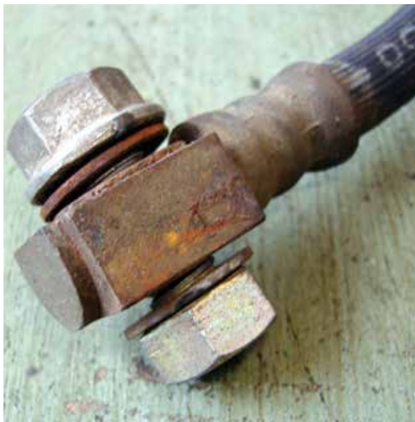
One way to block off a caliper for diagnosis is to use two copper washers and a nut and bolt on a banjo connection.
