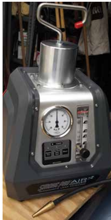
We know of no better way to find elusive intake tract leaks than with a smoke machine.
