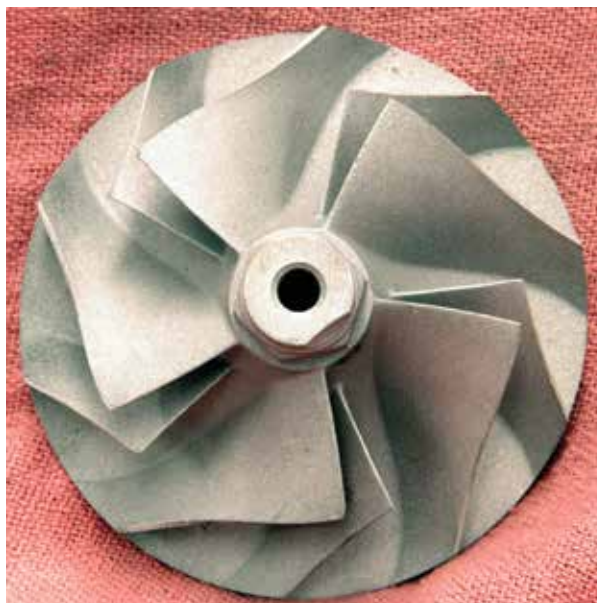
A whole lot of sophisticated engineering and manufacturing processes were needed to produce this compressor wheel.
