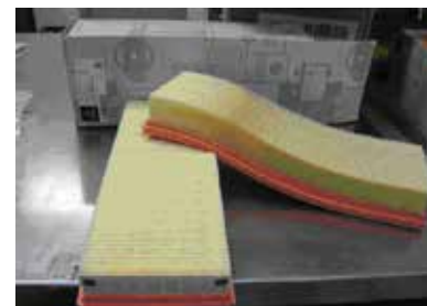
Before you start thinking about replacing a MAF sensor you're dubious about, look into the filter situation. If it's not a genuine Mercedes-Benz part, that could be the whole trouble.
