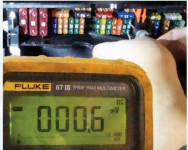
This test shows 000.6mV across the fuse which means there is an amp draw.
