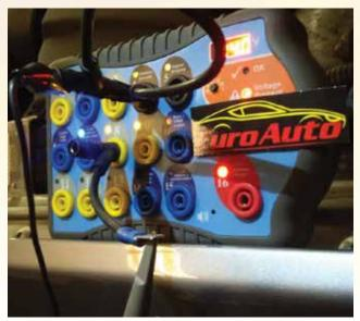
To view the actual network activity, a break-out box is used in between the DLC and diagnostic cable. Pay close attention to the LEDs when a diagnosis is performed on the entire vehicle or on a specific controller. My interest was pin 8 (K-BUS) and pins 6 and 14 (CAN-BUS).
