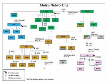
The use of data networks such as CAN Bus in vehicles has definitely simplified wiring and reduced weight, but it made diagnosis using only a wiring diagram nearly impossible. This shows the CAN networking used in the new Metris van, a relatively simple vehicle. To understand how a signal gets from here to there, you need to use the Function Diagrams found right next to the wiring diagrams in STAR Wiring and WIS.
