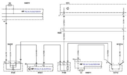
This section of the wiring diagram for the ECO Start system in a new Metris van (Model type 447) shows the auxiliary battery (G1/12) that powers the vehicle for the brief moment that the main battery is running the starter. Relay K120 switches the auxiliary battery on-line for that instant. Only a small part of the wiring diagram is shown here.
