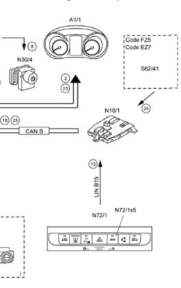
signal flow between and among components, particularly the signals on the CAN Buses (and other networks). If we want to understand where a particular signal starts from, or which signals are being received off the CAN Bus, we can turn to the electrical Function Diagram.
