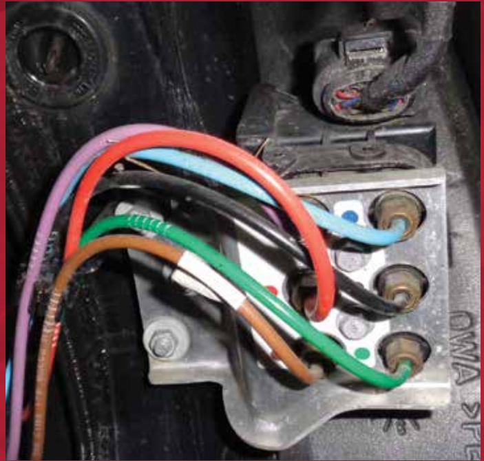
Air lines are color coded. Do not mix up line connections when servicing.
