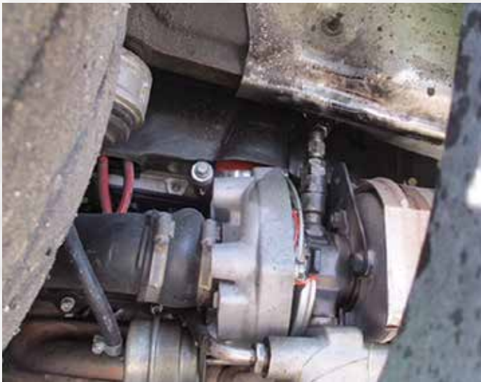
This turbo's impeller was lightened and balanced by someone lacking skills and equipment. The result was a total loss of the turbo itself. Note the pieces trying to escape from the housing.
