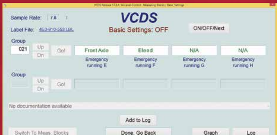
Running the bleed procedure will completely de-pressurize the front or rear axle separately to allow for safe repairs.
