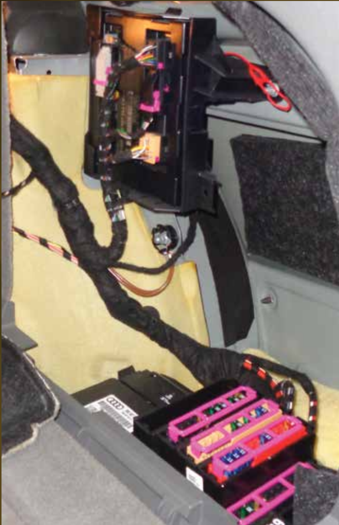
The vehicle battery and primary body control module are located in the right rear corner on this 2012 A4 Avant.
