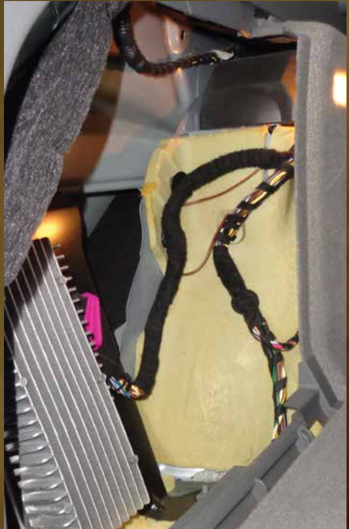
The audio amplifier location on an Avant model, located at the base of the C-pillar. This is prone to water ingress from clogged rear sunroof drains.
