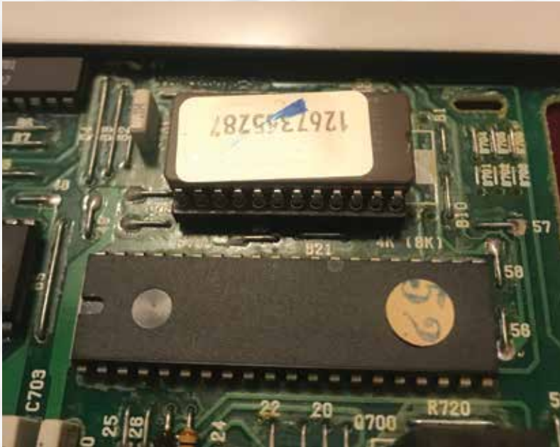
Replaceable and programmable EPROM sits in the brain and signals valves controlling the turbocharger.
