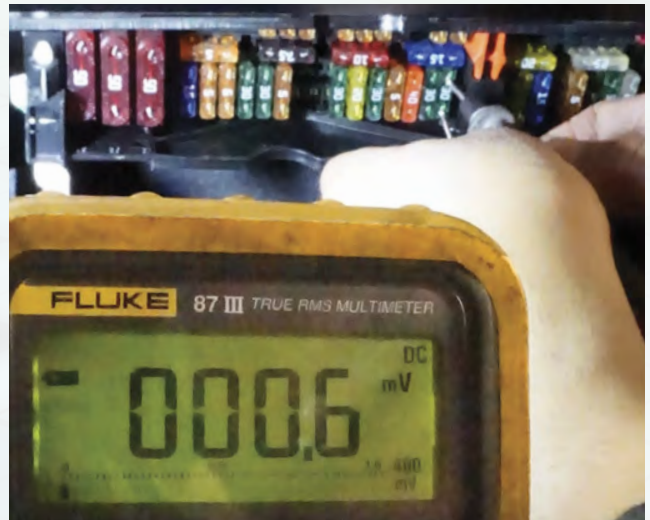
This test shows 000.6mV across the fuse which means there is an amp draw.
