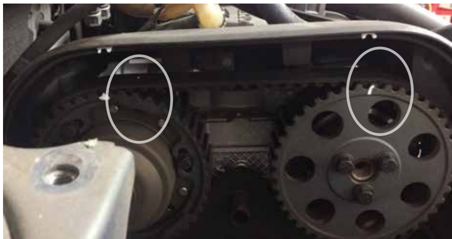
Here are the marks when lined up correctly.
