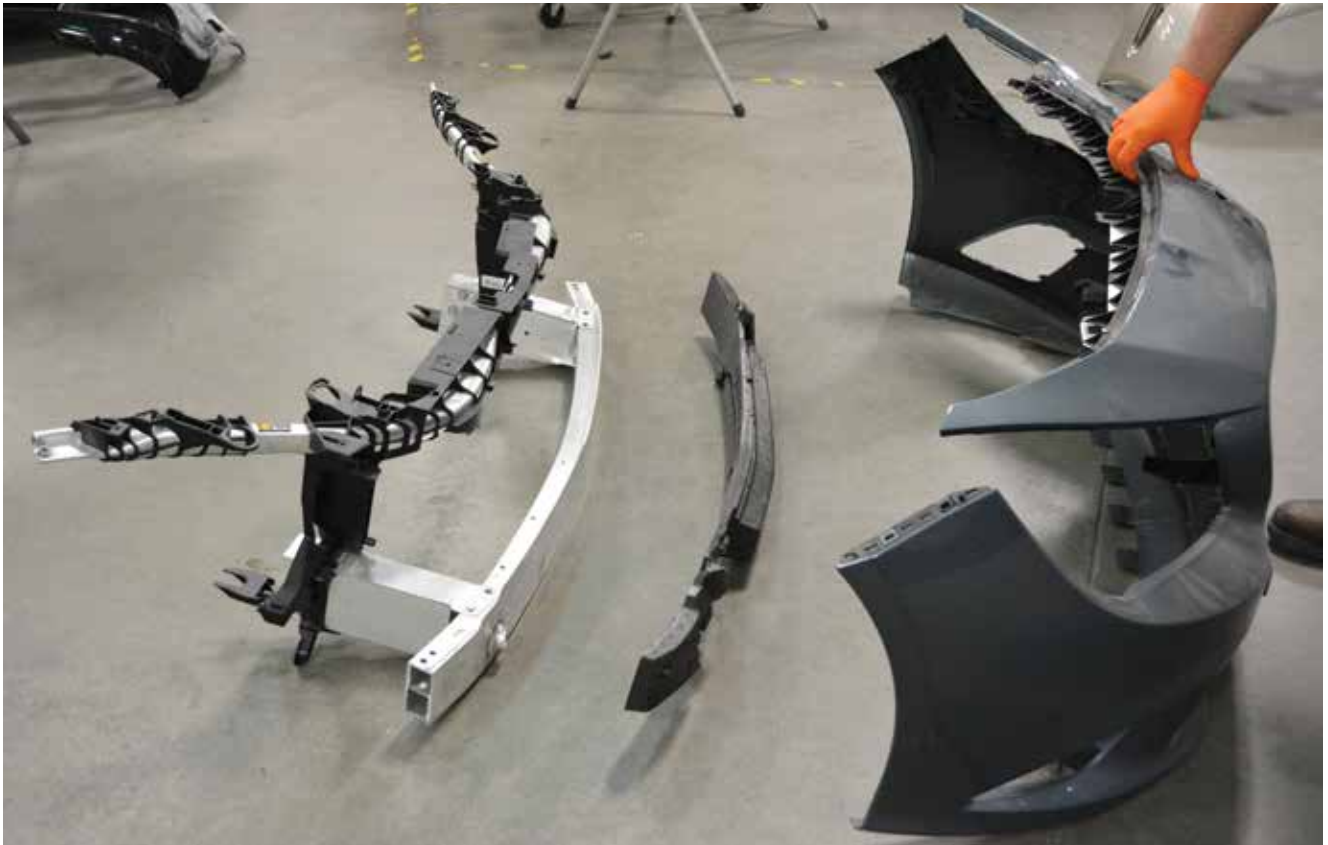
An aluminum reinforcement bar is built onto the crossmember of the front module. A foam impact absorber sits between the decorative bumper cover and the reinforcement bar.
