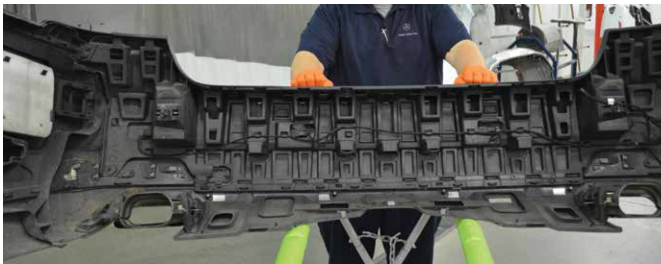
There are four Parktronic sensors in the rear bumper of this 2010 GL 450. Parktronic sensors in the rear help with lane departure warning and Parking Assist functions. There are similar sensors in the front bumper on many Mercedes-Benz models.
