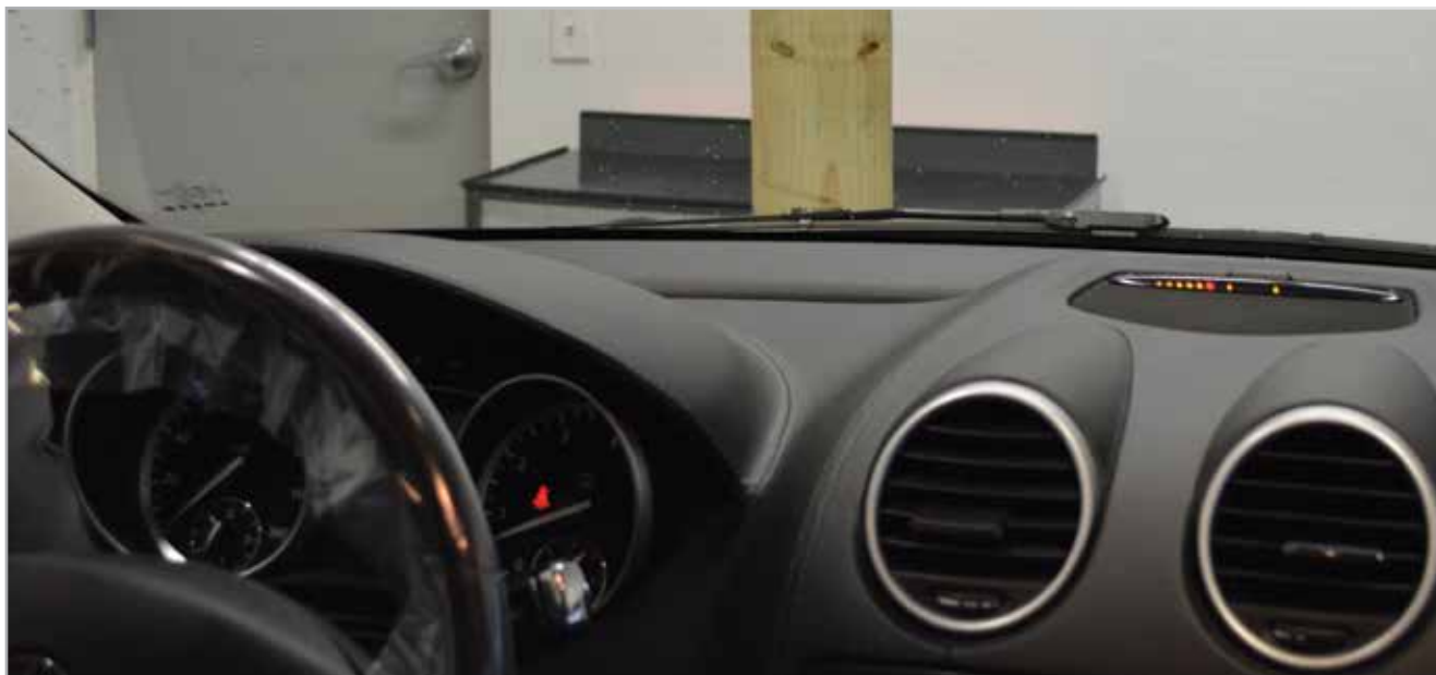
When it detects an obstacle (like the two-by-four stud we placed in front of this vehicle), the Parktronic system begins flashing red lights in two places on the dashboard.
