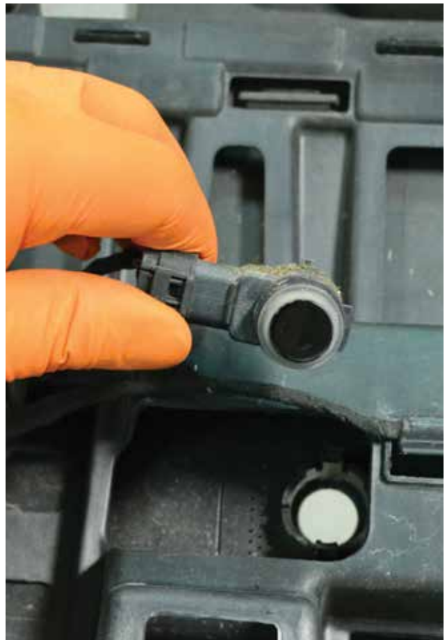
Mercedes-Benz short-range ultrasonic Parktronic sensors insert directly into the back of the plastic bumper, and include a seal that helps them resist road-induced vibration and shock.
