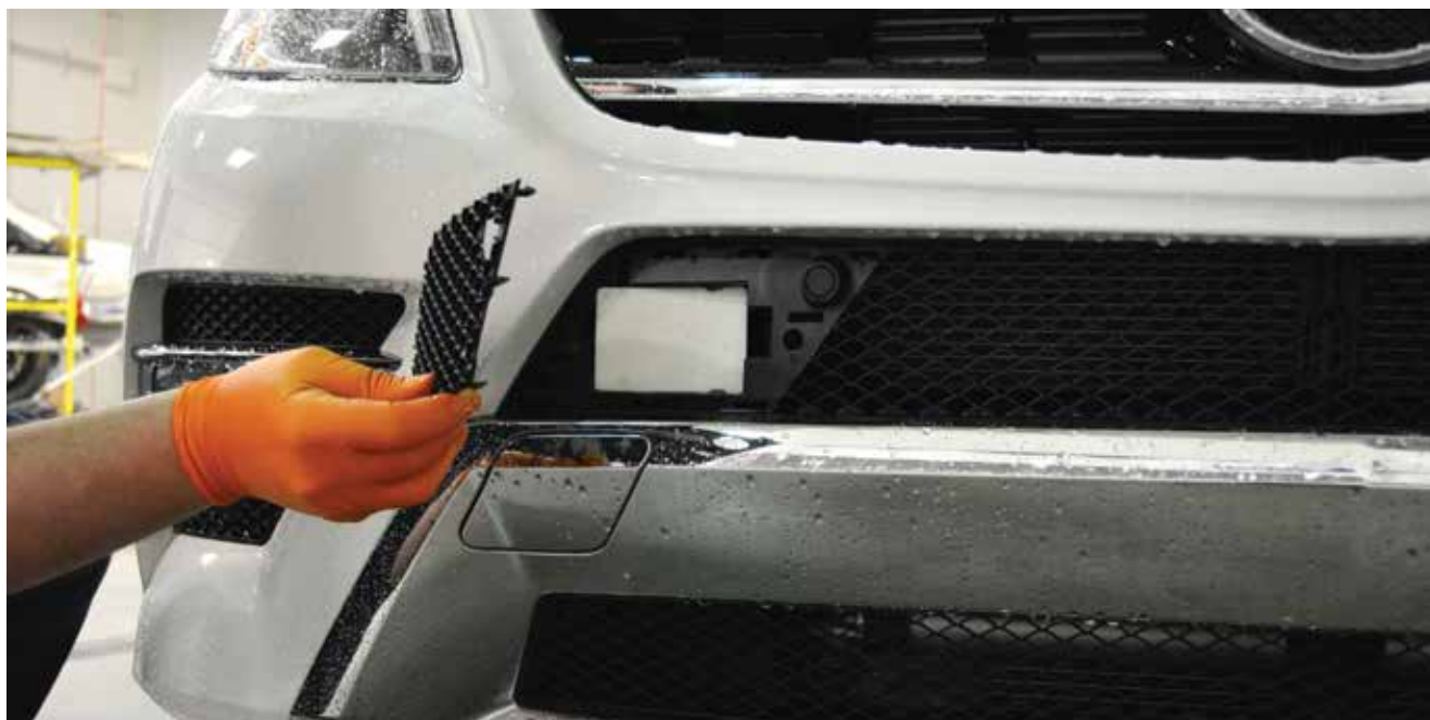
Collision avoidance sensors sit behind plastic grille covers in each side of the front bumper of this 2014 ML 350.
