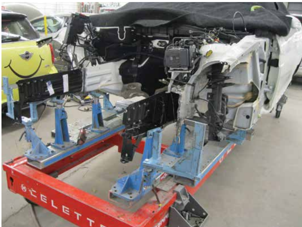
If a vehicle does not fit precisely in the fixtures of a Mercedes-Benz dedicated bench, it is a sign there is damage that has not yet been corrected.
