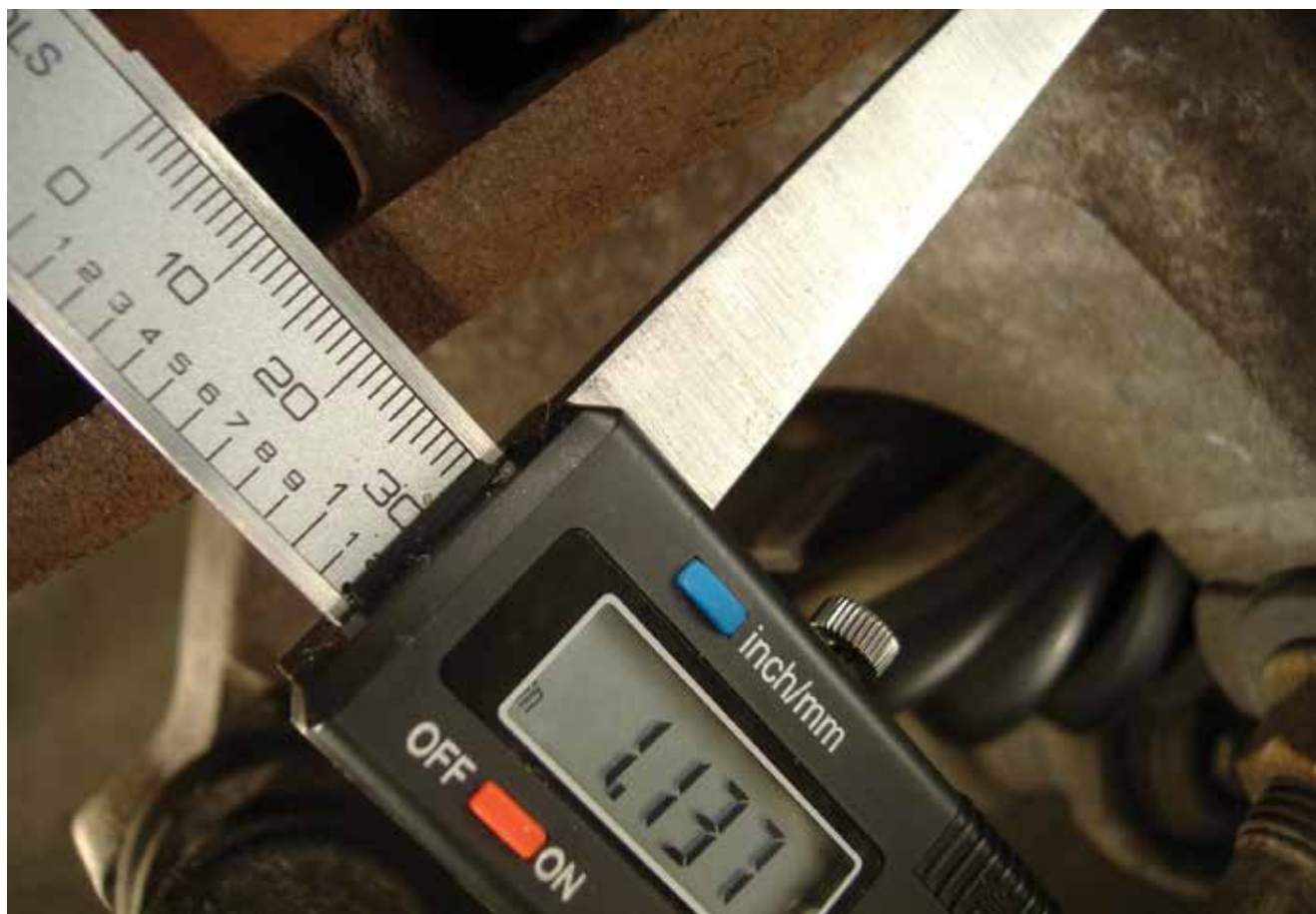
Our digital disc micrometer gives us fast readings, which we can use as a basis for rotor forecasting.
