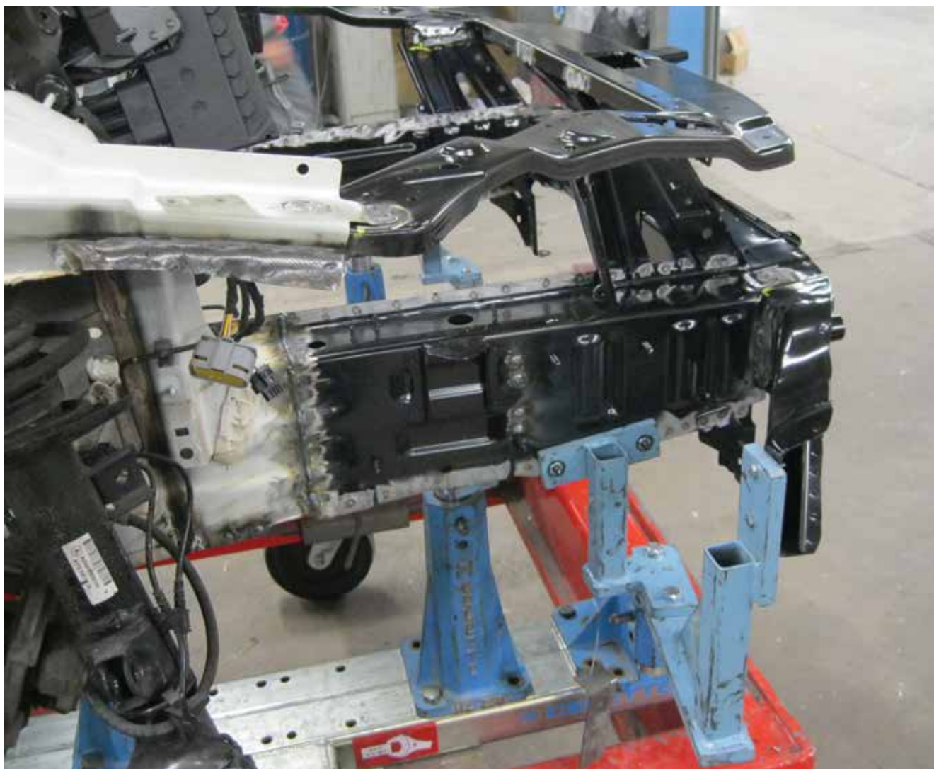
The Celette bench positions a structural member with factory precision, so it can be repaired with zero tolerance.
