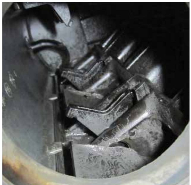
Looking inside this manifold, you can see the coked-up variable flaps, and also the vacuum line at the back coming from the internal reservoir.
