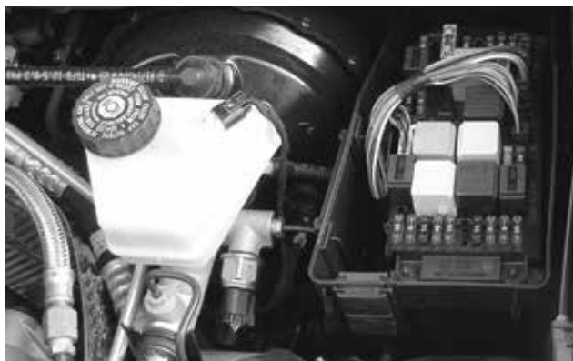
The driver's-side SAM generates a pulse width modulated (PWM) signal to tell the compressor control valve what refrigerant displacement level is needed for conditions.
