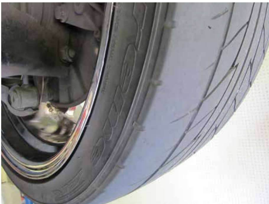
Here you can see tire wear and damage from an oversized wheel -- three inches larger than stock. This W220 also had heavy tie-rod wear/play from the sheer weight of the aftermarket rims.
