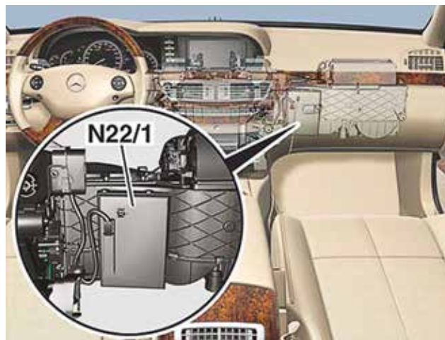
The ACC (N22/1) combines input from the dash controls with feedback from a variety of onboard sensors, and applies algorithms to make A/C function decisions that help Mercedes-Benz vehicles maintain their fuel-sipping attributes.
