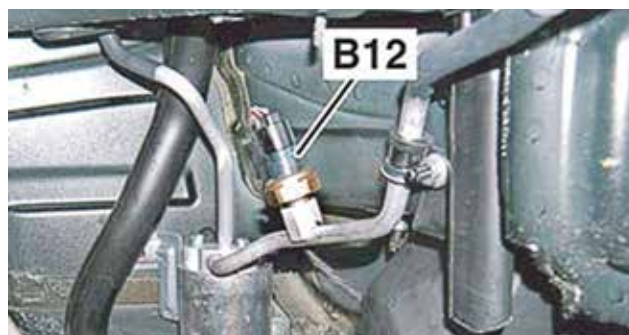
Various refrigerant pressure sensors provide input that's used to make the displacement decision.
