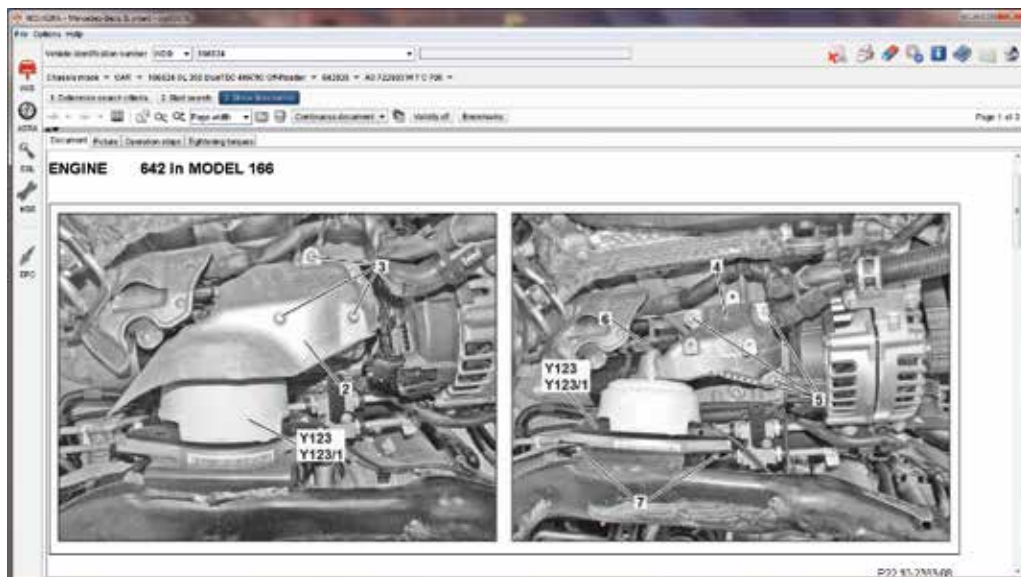
These modern motor mounts are still serviced in the same way as a conventional unit with the minor exception that there is an electrical connector to unplug. With your paid subscription to www.startekinfo.com , you can access WIS and get a step-by-step procedure for diagnosing and replacing the new mounts.
