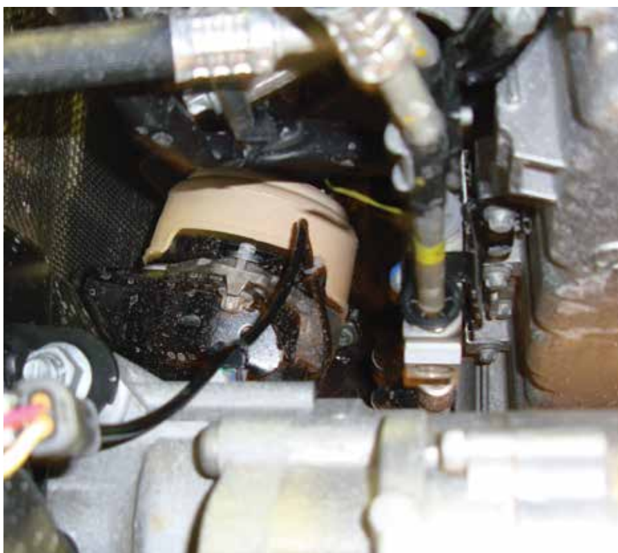
The two-wire harness is a surefire give-away that this is a computer-controlled mount. It is powered up by fuse F58. If you unplug the fuse and plug it back in with the key on, you should hear the mounts click.
