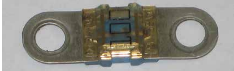
This blown 100A fuse was hidden in a front SAM unit.
