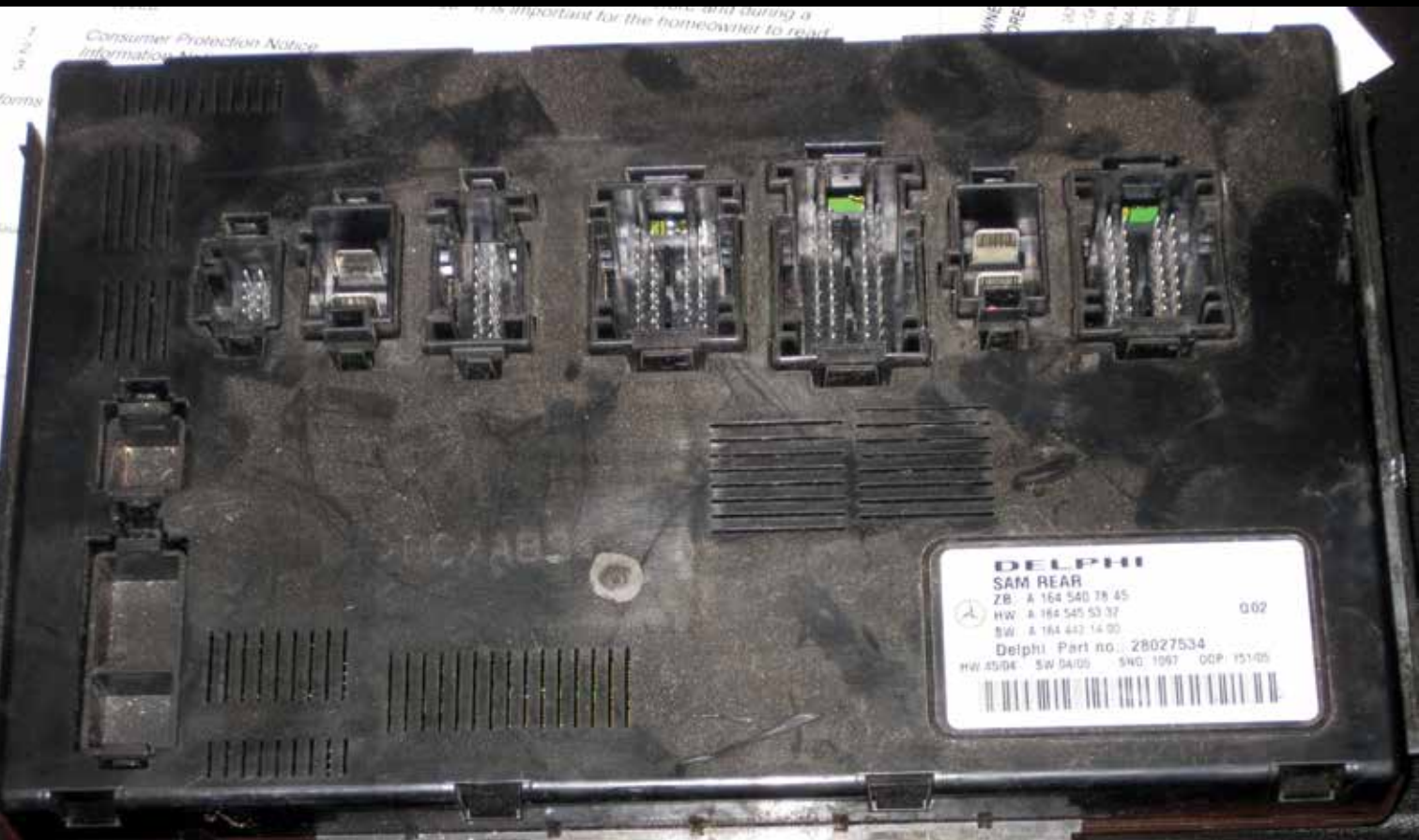
This rear SAM has seven multi-connectors, but XENTRY makes it easy to identify them.
