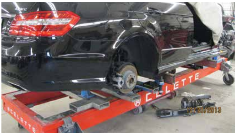
The Sevenne XL Bench from Celette is Mercedes-Benz approved when used with the Mercedes-Benz Anchoring Kit, plus aluminum crossmembers that accept the appropriate fixture sets. Image courtesy of Reliable Automotive Equipment ( raeservice.com ).
