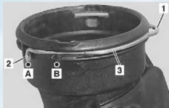
This spring clip holds the air filter hose to the rest of the intake. To remove the hose, slide the spring nose from (A) to (B). Never pull on the eyelet (1) or you'll damage the spring.
