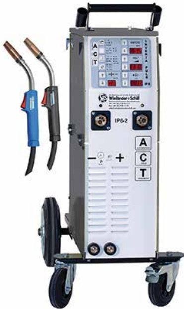
The Mercedes-Benz approved InvertaPuls IP6-2 aluminum welder from Wielander & Schill uses inverter-based pulsed MIG welding technology. Inverter technology allows the flexibility to adjust equipment settings and welding technique to reduce burn-through and distortion when welding aluminum or thin sheet steel. Image courtesy of Reliable Automotive Equipment (raeservice.com).
