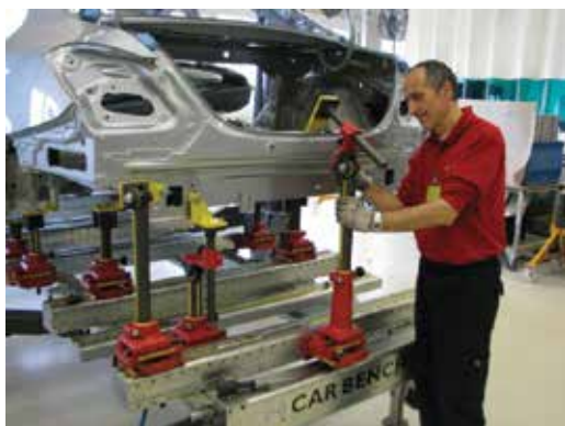
The jig setup for straightening this Mercedes-Benz C-Class may differ from the fixtures required for a Mercedes-Benz model built on a different chassis. Image courtesy of Car Bench.
