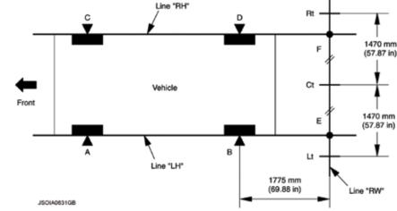
Once you set up the targets and input the rear view camera height to your CONSULT III Plus, select "Rear Camera ITS" and press "Start." CONSULT III Plus will take you through the process of aiming and verifying the camera calibration.
