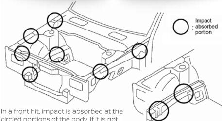
circled portions of the body. If it is not absorbed completely, impact damage can travel to the dash panel and roof.
