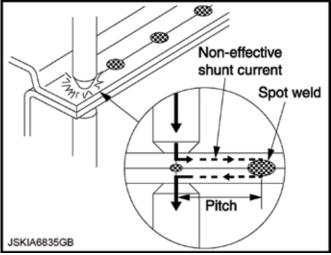
The BRM-Fundamentals manual explains the general principle behind the recommendation to avoid an excessively small pitch between spot welds (inadequate pitch allows current to flow to the nearest welds, reducing weld strength).
