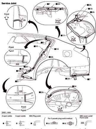
In one image, Nissan shows a large amount of information needed to replace the rear fender on a 2012 Altima sedan. It includes cut locations for replacing the fender, and explains that the cuts are MIG seam welded, that MIG plug welds are used in many other areas of the repair, that many are 3-panel thickness, and that almost all are plug welded from one side only. The key across the bottom of the image shows symbols that represent each different weld type used in the repair.
